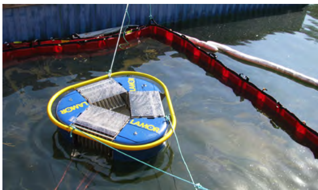
Figure 7. The MultiSkimmer with disc modules demonstrated its recovery capabilities with light oil, in a manner similar to that of other disc skimmers. Photo: Manu Kettunen, 2025.
