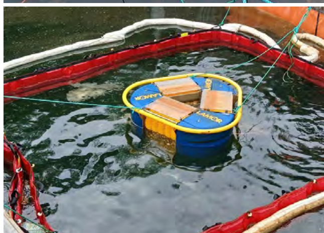
Figure 6. A foamy emulsion formed when collecting with the brush module. However, 90–95% of the oil was removed. Photos: Manu Kettunen, 2025.
