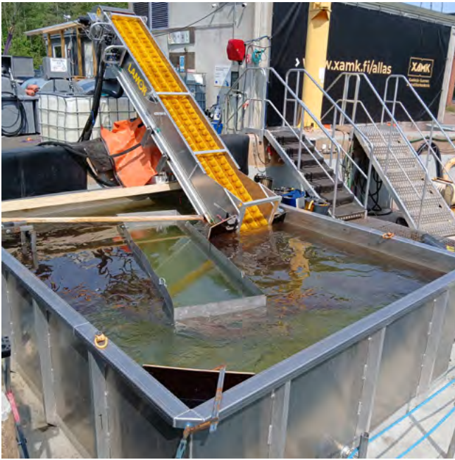
Figure 3. The flow conditions required for the bow collector were achieved using deflection plates and a hydraulic flow propeller. Due to the structures, the oil surface area was reduced to approximately ten square meters. Photo: Justiina Halonen, 2025.
