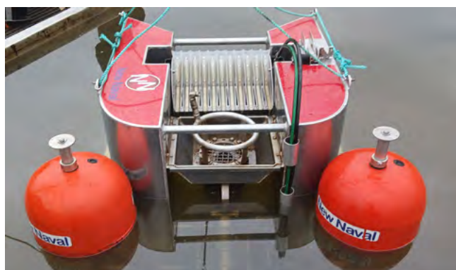
Figure 14. ScorSkim 30 equipped with a disc module. Photo: Justiina Halonen, 2025.
