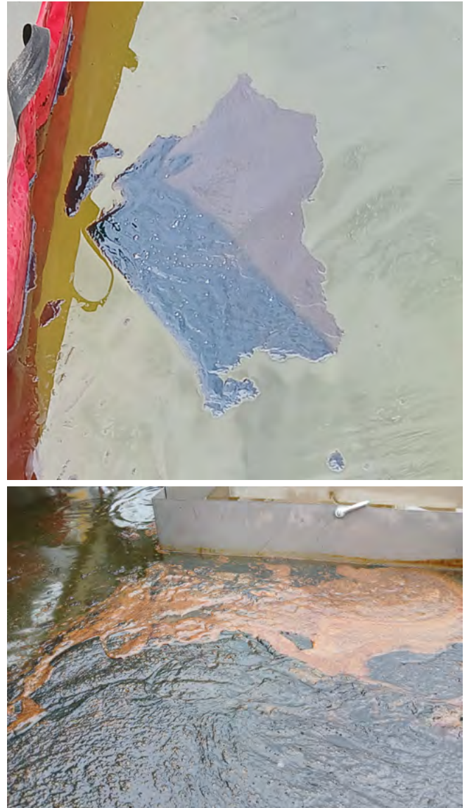
Figure 10. In the shaded area, the ultra-low-sulphur fuel oil (RMD80) remained fairly thick. The part of the oil slick exposed to sunlight warmed up and thinned out. This difference is visible in the portion of the oil slick partially shaded by the boom. Water temperature: 16°C. Photos: Justiina Halonen, 2025.
