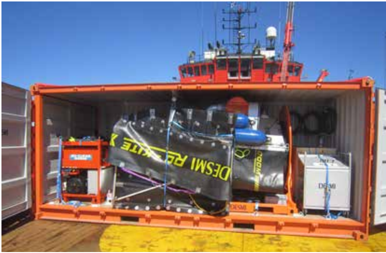
20" Container comprising of 50kW Power Pack, DESMI Speed-Sweep 1500 and Guide Boom, ZUH-hose on Reel, Ro-Skim 1500 and Ro-Kite 1500.
