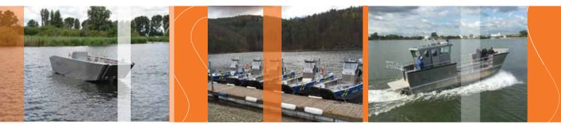
DESMI is concentrating on landing craft type of aluminum boats due to versatility and easy access for equipment placed on the boat. As a standard DESMI is promoting the following sizes:
