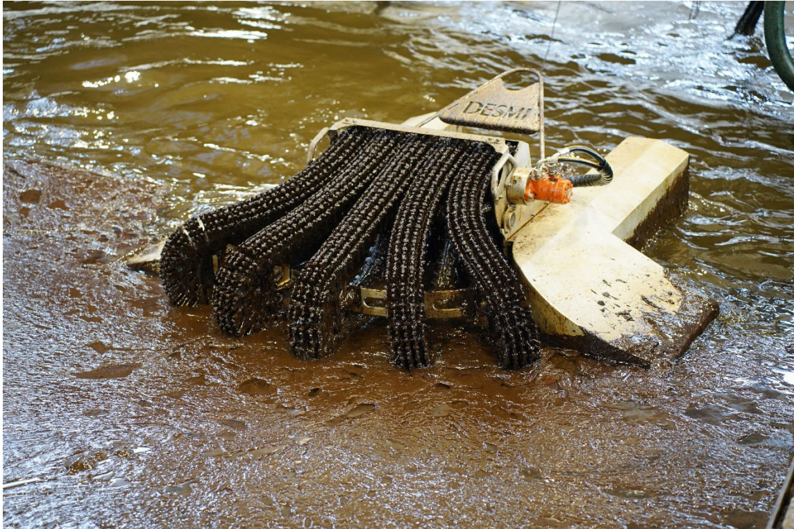
Figure 6: Photo of the DESMI modified Octopus skimmer operating in the IM-29 oil.
