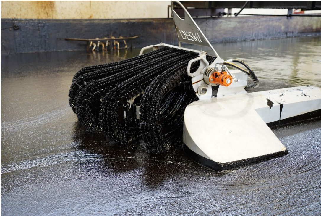
Figure 4: Photo of the DESMI modified Octopus skimmer operating in the IM-27 oil.
