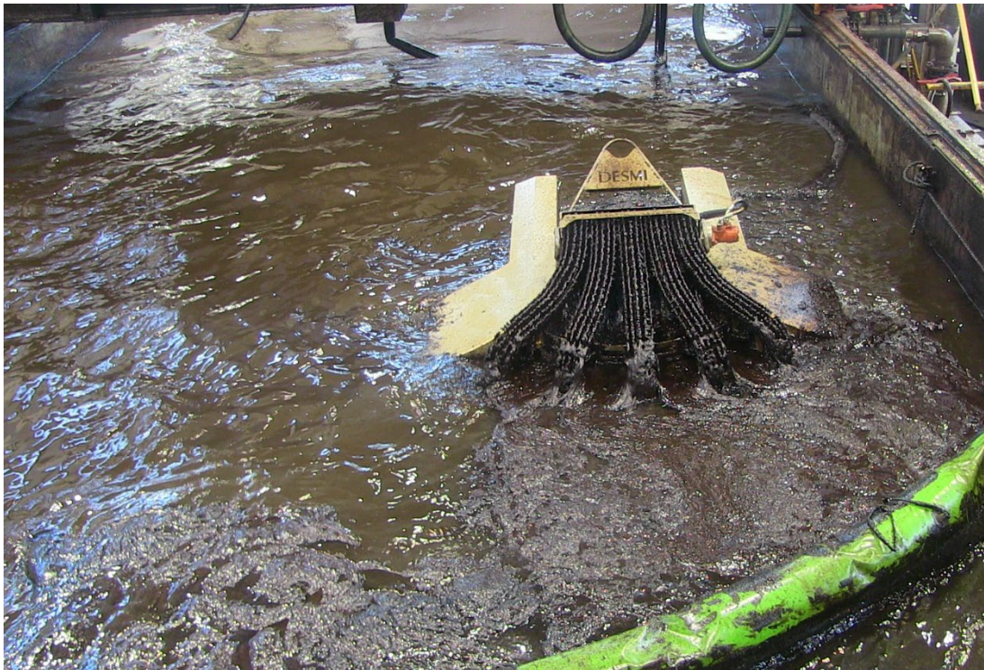
Figure 5: Photo of the DESMI modified Octopus skimmer operating in the IM-28 oil.
