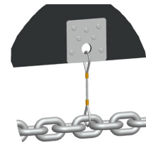
Chain connected to boom by wire
